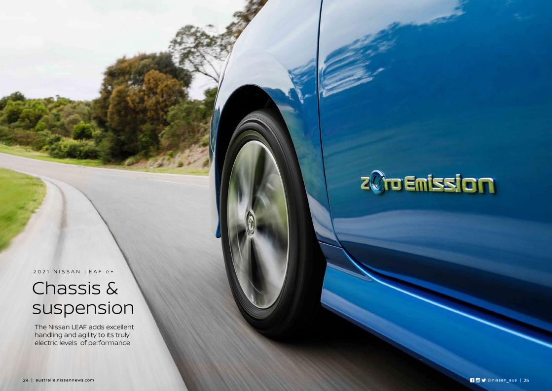
he Nissan LEAF and LEAF e+ prove that efficiency need not come at the cost of driving excitement. Heavy components, including the battery, are placed in the centre of the body – lowering the centre of gravity by five per cent over the previous generation LEAF — helping achieve smaller yaw moments of inertia compared with front-engined vehicles, and thereby improving directional stability and enabling smoother cornering.
