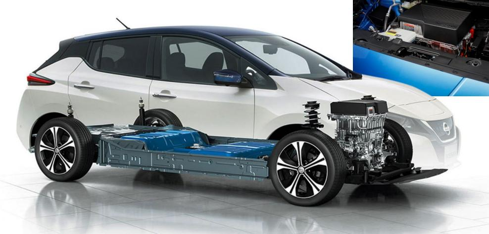
he e-powertrain delivers an exhilarating, linear driving performance, with a power output of 110kW for the LEAF and 160kW for the newly released LEAF e+.
